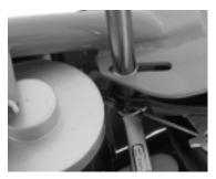
Fig. 16. Loosen brake housing anchor and disconnect.
